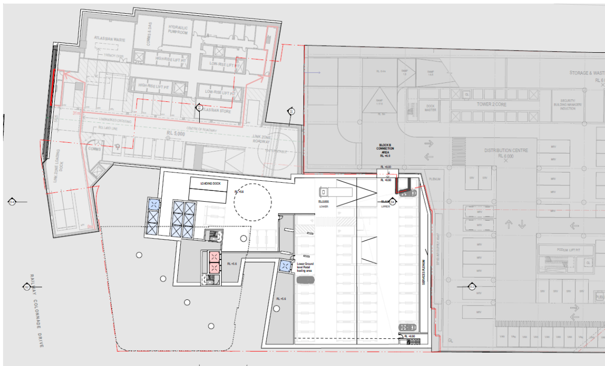
Figure 4.5: Indicative upper basement parking and loading
