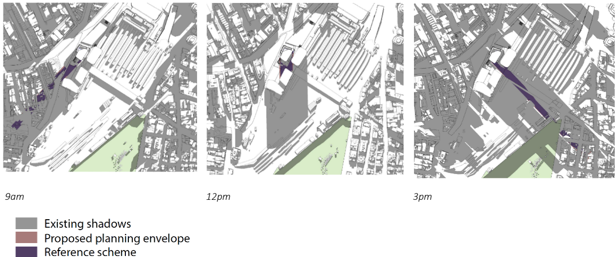
Figure 43. Shadow Analysis of Block C building envelope on 21 June
