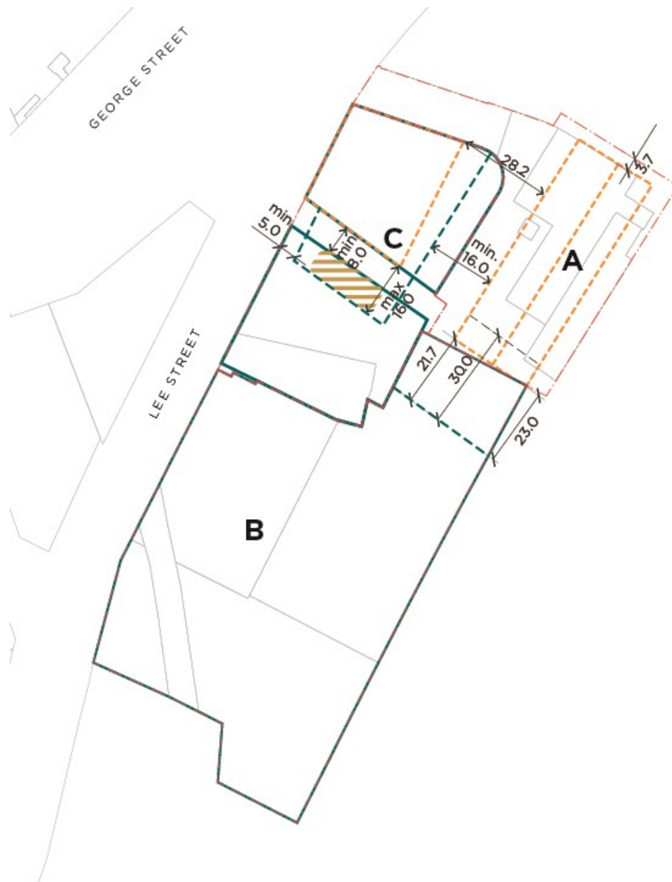
Figure 41. Building Envelopes, separation distances and setbacks
