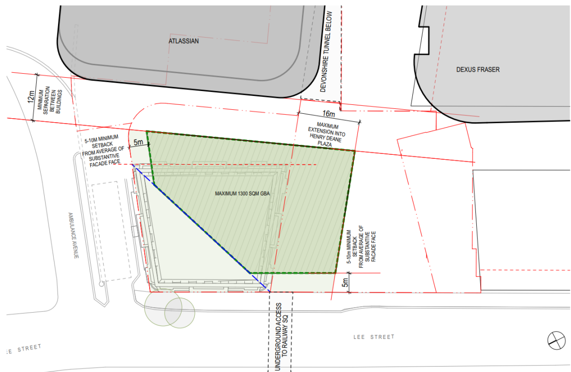
Figure 33. Building footprint and separation
