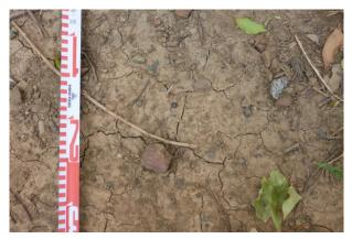
Picture 95 – Detail view of dry, tightly packed clay subsoil with in an exposure
