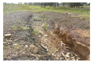
Picture 96 – Exposed, disturbed clayey subsoils with ironstone gravels within the northern portion of the Study Area and along a vehicle access track
