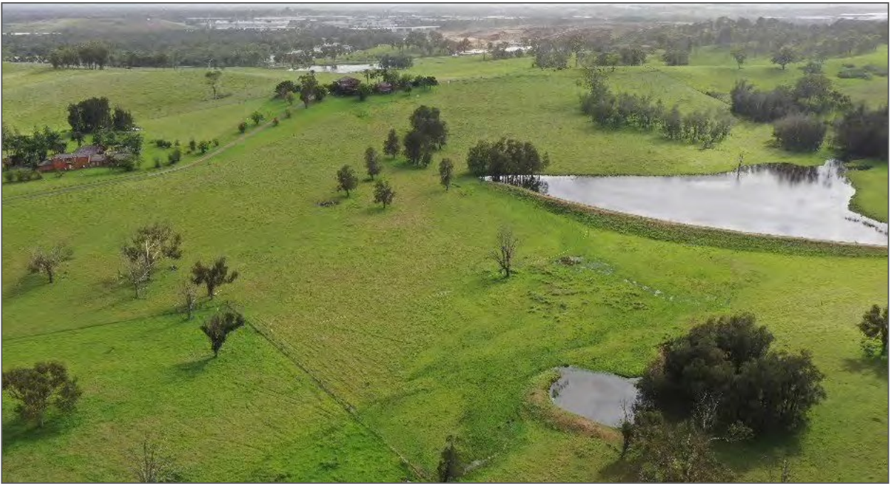
Figure 15: Mid-section of watercourse with large farm dam. Overland flow path is evident on downstream side of dam.
