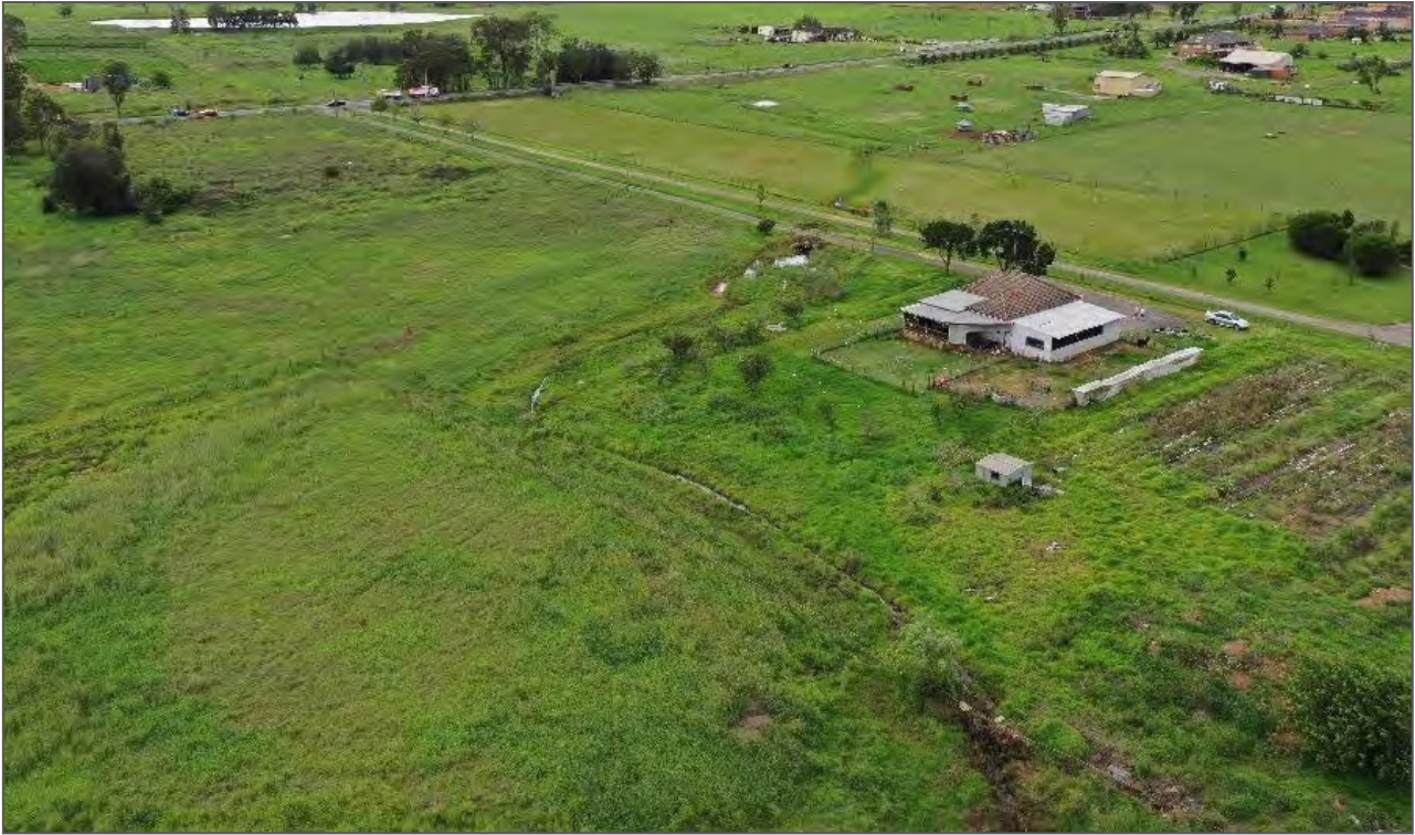
Figure 17: Lower section of Unnamed Trib South Creek 1. Channel modification and erosion is evident.
