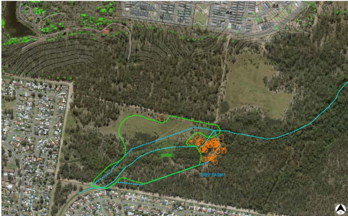
Figure 10: Detailed view of the existing (blue) and proposed (green) Drainage Basin I.
