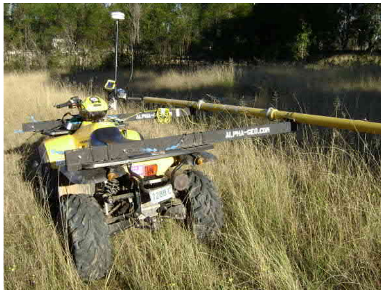
Photo 3 – DualEM-4 mounted on ATV
