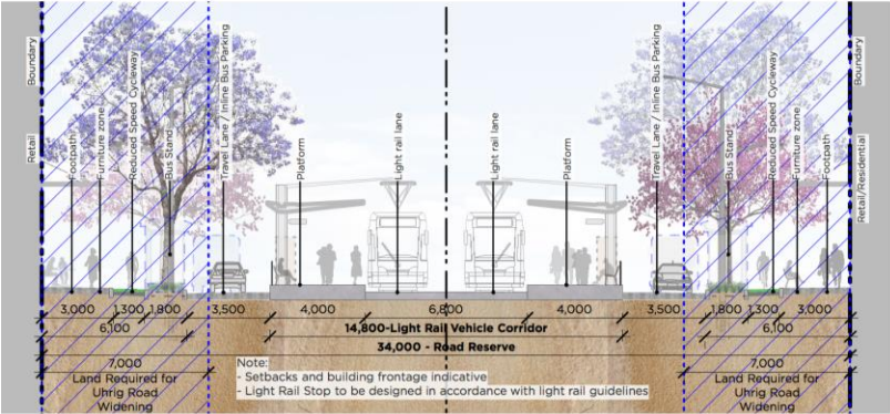
Uhrig Road North Typical Section
