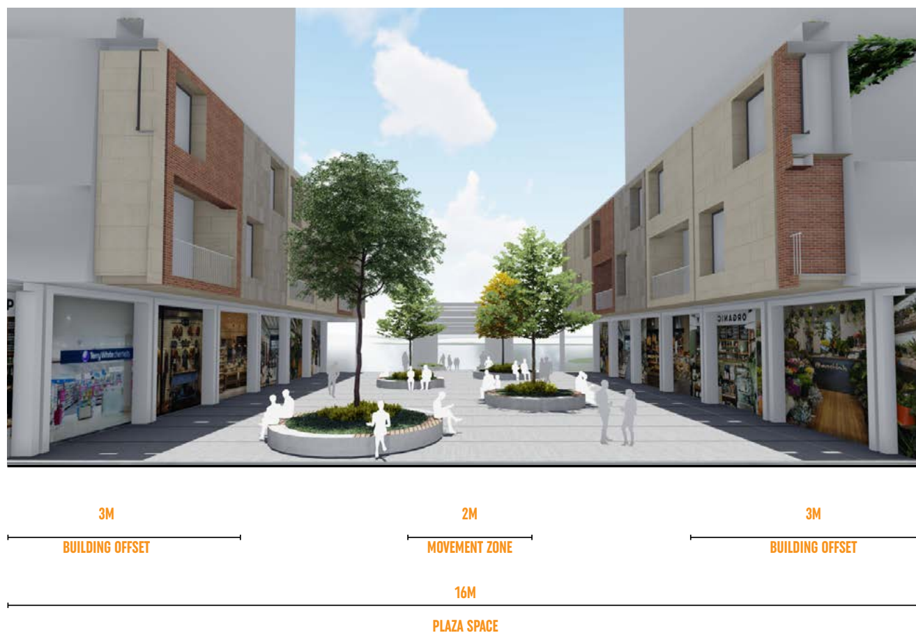
Figure 194. Bridge Plaza Cross Section
