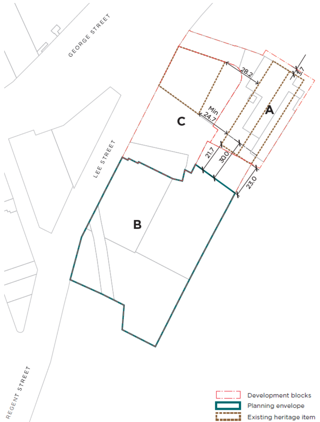
Figure 3: Separation distances and setbacks – Lower Level
