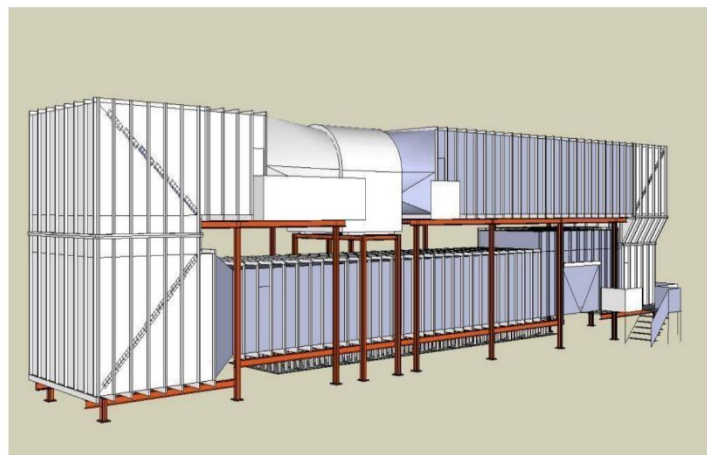
Figure 1: Schematic of the closed-circuit wind tunnel.
