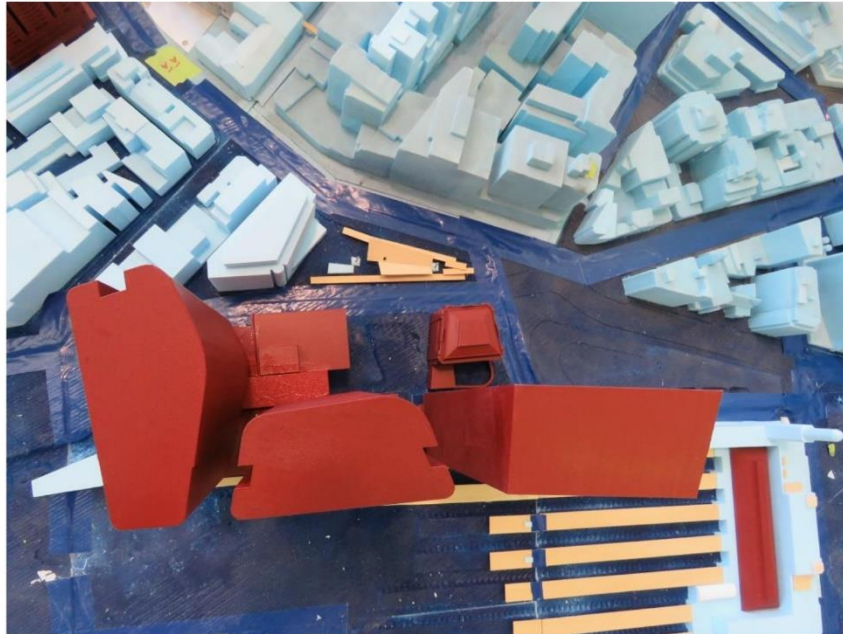
Figure 10: Close-up of the wind tunnel model in Configuration 1 viewed from above.
