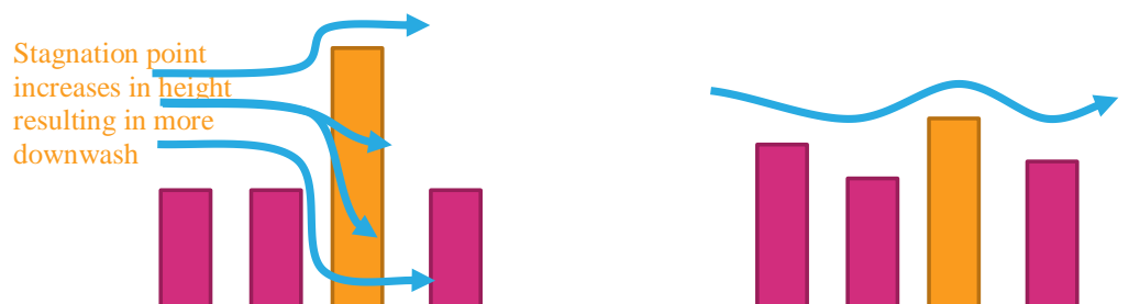
Figure 16: Schematic of flow pattern interference from surrounding buildings
