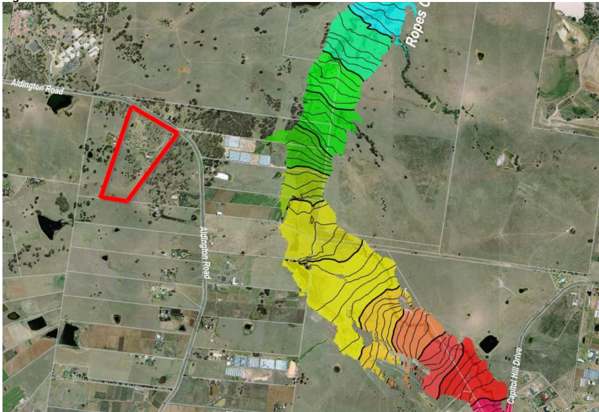
Figure 7 – The Site - Probable Maximum Flood Extents
