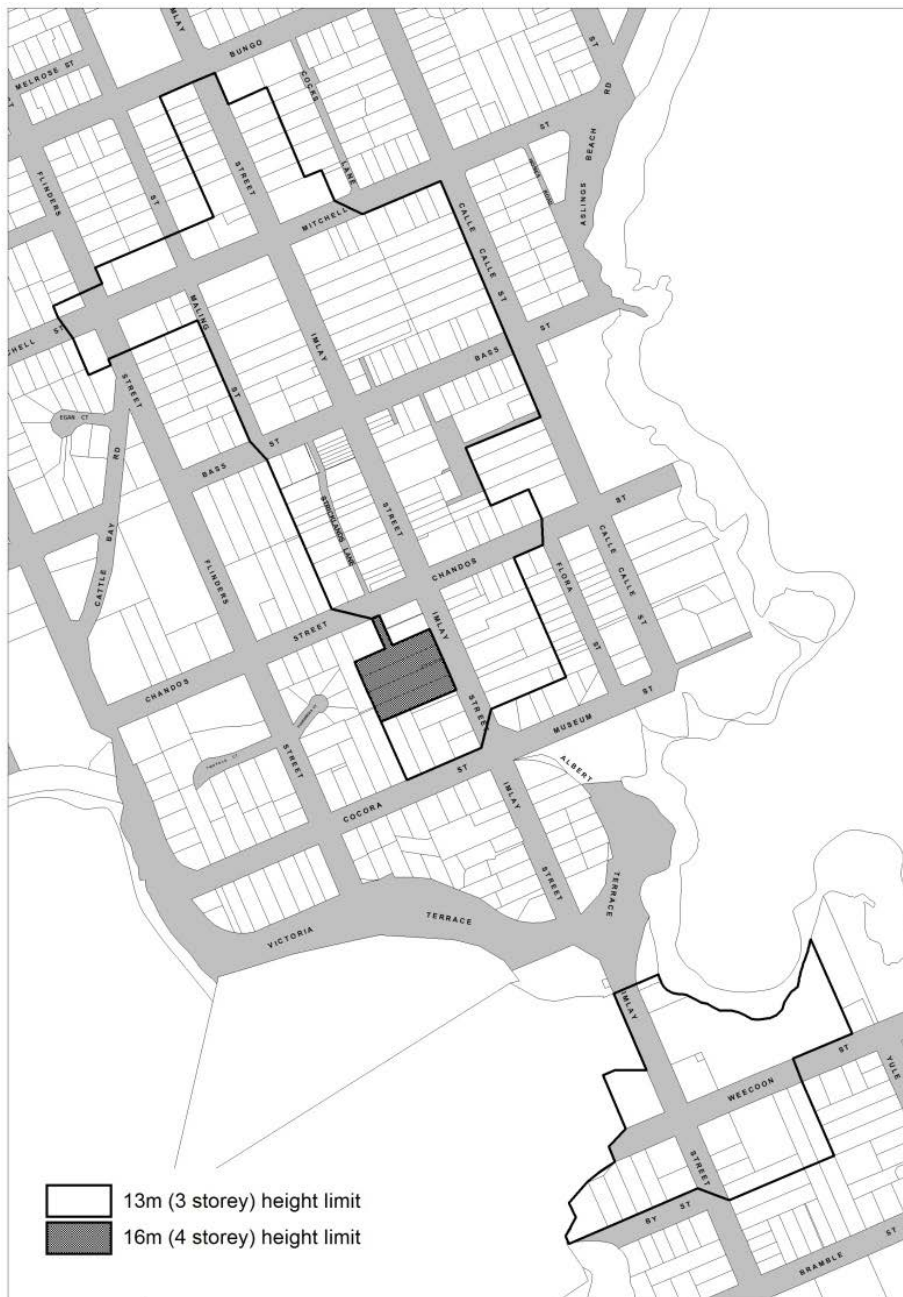
Figure 2.5 Eden building height limit
