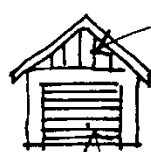
SIMPLE GABLE TREATMENT DOORS TO BE SIMPLE TIMBER OR METAL CLADDING - NOT PANELLED 'FANCY' DOORS
