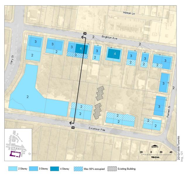
Figure 8 - Block B Control Plan
