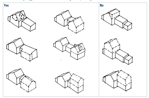
FIGURE 3 Single storey housing – principal building form shown hatched
