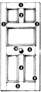
Some common examples of front doors are shown. All are panelled doors with stiles and rails. Type A and Type B are four panel doors, while Type C is a high-waisted Edwardian door.
