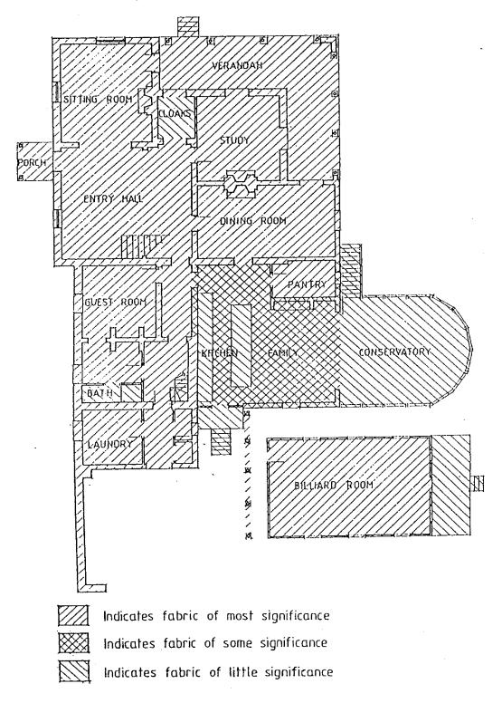
FIGURE 2 Plan of first floor indicating significant fabric
