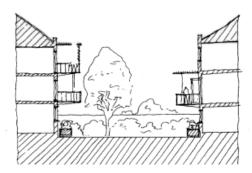
**FIGURE 48** Vegetation and balcony screening must be used to enhance privacy when the recommended separations are not able to be achieved.
