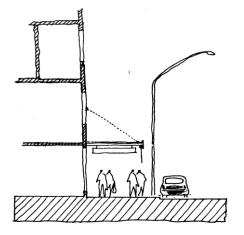
FIGURE 1 Awning design – suspended steel box section type with a minimum soffit height of 3.2m
