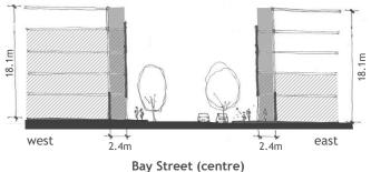
Design colonnades including the size and spacing of the columns integral with the building design and with regard to adjoining colonnades if they exist
