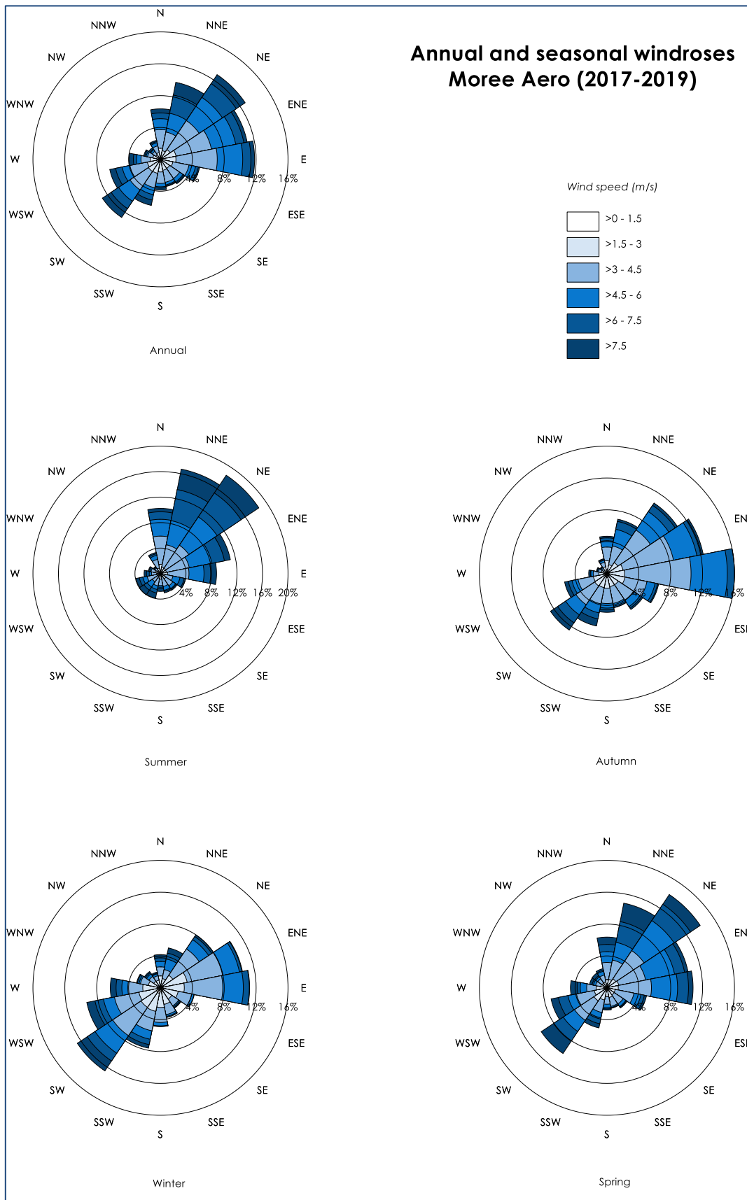
Figure 3-3: Annual and seasonal windroses showing meteorological conditions for Moree Aero, 2017 to 2019.
