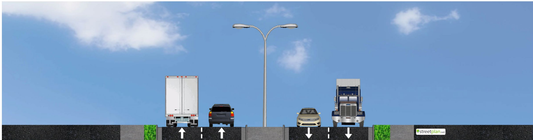
Figure 7-2 Major arterial and spine road cross-section
