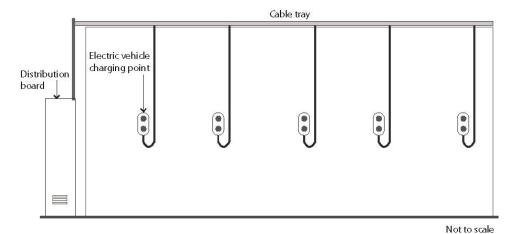
**Figure 2:** Electric vehicle charging points and electric circuitry provision in development with multiple car spaces using buried underground cable system.
