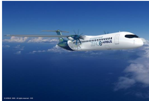
Fig 17: Propeller plane driven by fuel cells
